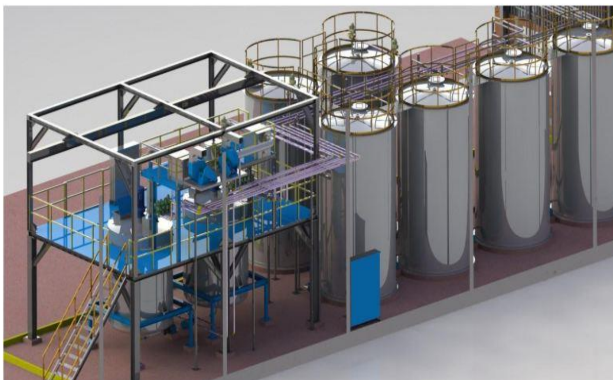
Figure 4. 5 Small Modular 3D Admixture Plant Design
